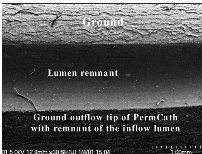
Fig. 9 - Ground outflow tip of the PermCath™. The remnant of the inflow lumen is smooth, whereas the ground surface is rough.
