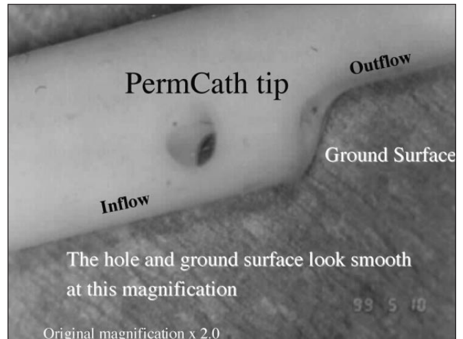
Fig. 2 - Higher magnification of the PermCath™ side hole and ground outflow tip. Both the holes and the outflow tip look smooth at this magnification.
